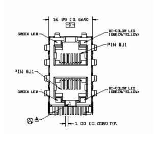
Figure 12. Stacked Ethernet Connector
